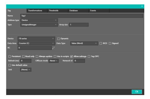
The Tag addressing is physical based on the PLC memory mapping.
