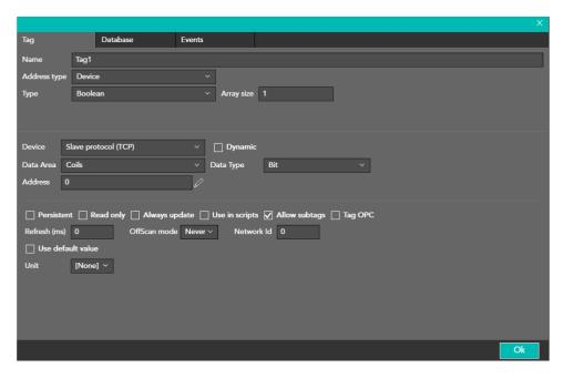
Modbus slave variables are variables available for the Master which has to read and write them. The HMI panel never takes the initiative and responds to requests from the master.
